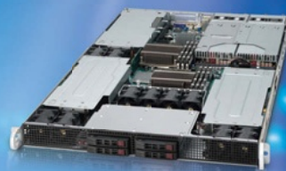
1U 4 GPU Server SYS-1022GT-TRF-FM407 • 2 TFLOPS (Double Precision)
