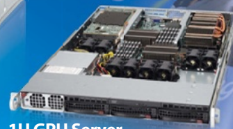
1U GPU Server SYS-6016GT-TF-FM207 • 1 TFLOPS (Double Precision)
