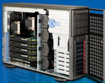
PSC: Personal Super Computer SYS-7046GT-TRF-FC407 • 2 TFLOPS (Double Precision) in 4U
